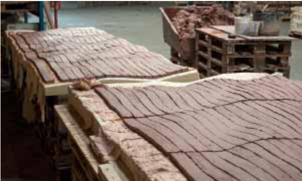
8. The clay elements are placed on the polyurethane moulds, ready for drying
