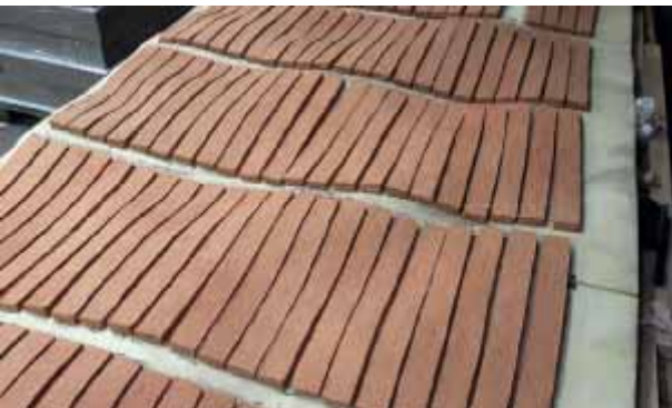
10. The brick elements are placed on the moulds.
