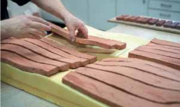
2. Inspecting the first sample brick after firing.
