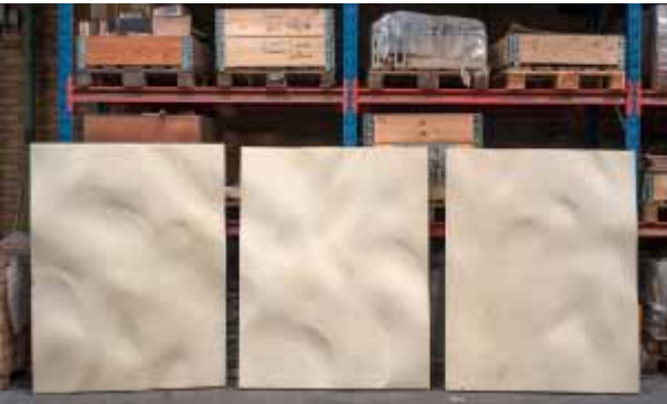
4. The finished mould is ready for the clay elements.
