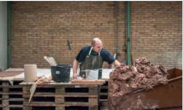
6. The kneaded clay is ready to be shaped.
