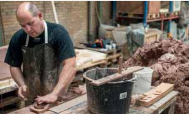
7. The clay is pressed into the wooden moulds.
